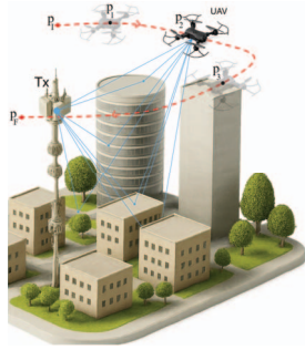
Fig. 1: Efficient radio mapping of inaccessible regions using optimized UAV trajectory measurements
