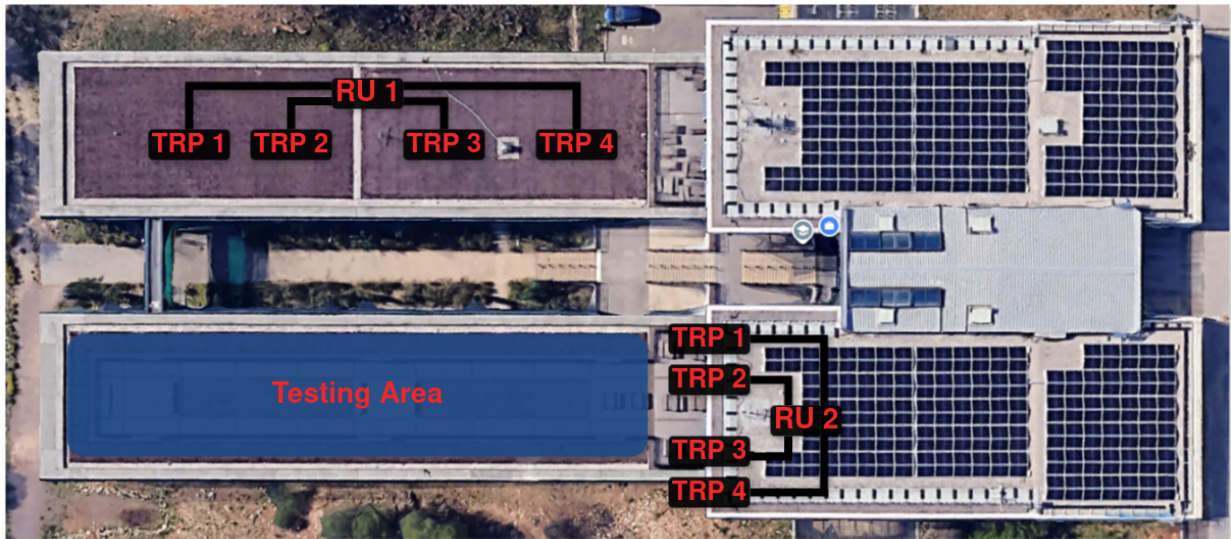
Fig. 14: GEO-5G testbed: Deployment of 2 O-RUs each with 4 distributed TRPs on the south terrace and the north rooftop of EURECOM, with a testing area of size 50x10 on the north terrace
