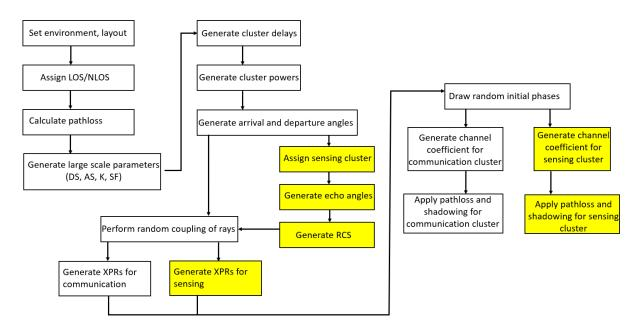
Figure 1. Channel coefficients generation procedure for communication and sensing channels.
