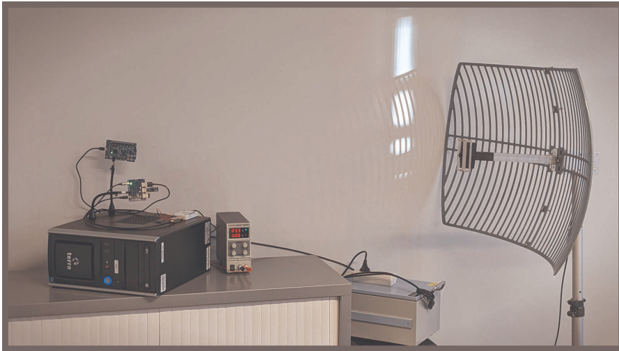
Figure 5.4: Collection setup using the directional antenna.
