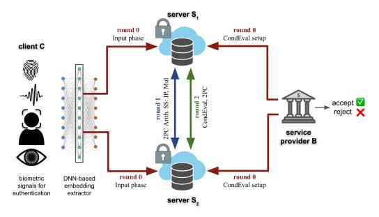
Figure 1: Privacy-preserving biometric authentication system based on cosine similarity in the 2PC setting.
