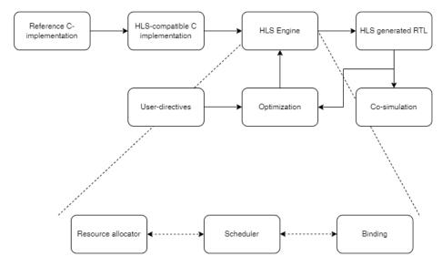
Fig. 2: A highly simplified overview of the HLS flow. Adapted from [17]
