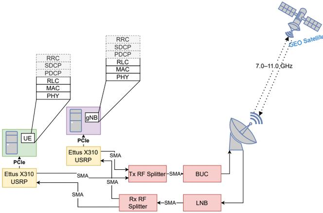
Fig. 6. 5G NTN architecture (*noSI* mode) for the field trial. Our demonstrator includes adapted PHY, MAC, and RLC layer for OAI.
