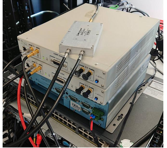
Fig. 8. Two Ettus X310 USRPs functioning as both the gNB and the UE in the NTN demonstration.
