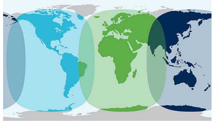
Fig. 1. Three GEO satellites can almost cover the whole globe [13].
