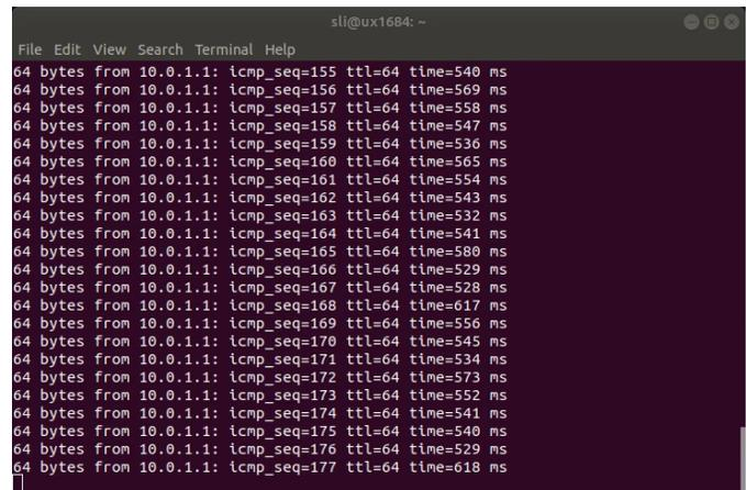
Fig. 11. Measurement of the RTT between UE and gNB with ICMP messages.
