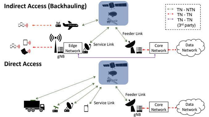
Fig. 2. High level 5G NTN architectures for the indirect access (backhauling) and the direct access. The direct access architecture utilizes the NR waveform on both, feeder link and service link. A direct access UE is sending data over the SatCom link without relay in between.
