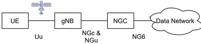
Fig. 5. 5G NTN architecture for direct access including UEs, a transparent satellite link, a gNB and the 5GC.
