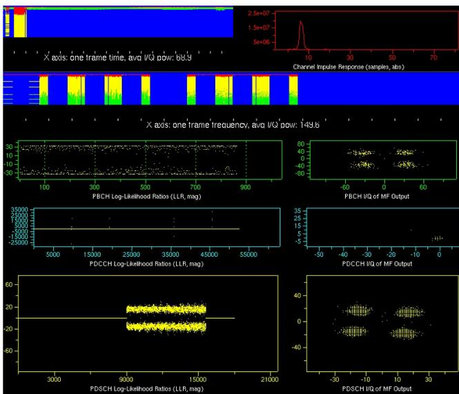
Fig. 10. OAI GUI: QPSK constellation diagram of PBCH (top right) and the PDSCH (bottom right) at the NTN UE.
