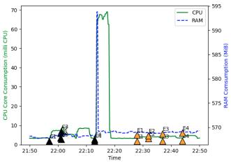
Fig. 7: Computational Resource Consumption for 4 Edge Slices
