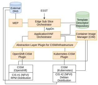
Fig. 4: Lightweight edge Slice Orchestration Framework
