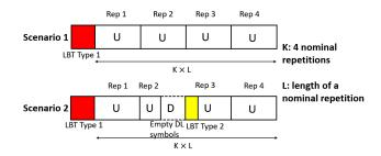
Fig. 2. UL transmission in TDD configuration unlicensed spectrum.
