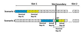
Fig. 3. Interruption in the transmission of UL repetitions due to orphan symbol in unlicensed spectrum.
