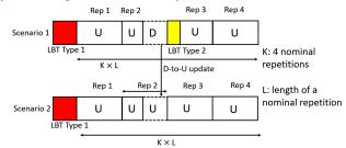
Fig. 4. Semi-static DL symbols are switched to UL symbols.
