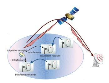
Fig. 1. FS based systems receiving interference from satellite systems.
