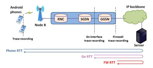
Fig. 1. Measurement setup.
