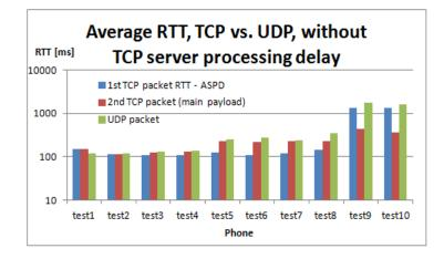
**Fig. 3.** TCP vs. UDP latency: average recorded RTTs, with average server processing delay subtracted from the 1<sup>st</sup> TCP packet RTT, logarithmic scale.
