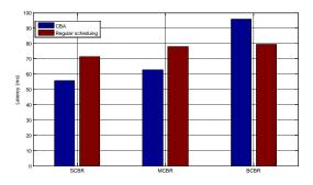
Figure 2: Measured latency using OAI for contention-based uplink channel access (targeted towards machine-type communication) relative to regular scheduling under three different traffic patterns: small packet CBR (SCBR), medium packet CBR (MCBR) and big packet CBR (BCBR).
