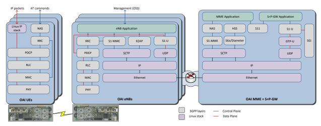
Figure 1: OpenAirInterface LTE software stack over ExpressMIMO2 software radio frontend.
