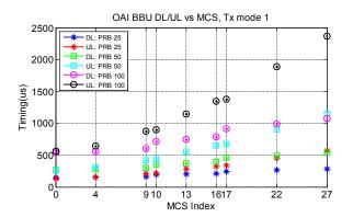
Figure 3: Results of profiling OAI baseband functions from a C-RAN perspective.
