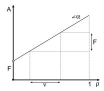
Figure 1: Linear power consumption model for a link.
