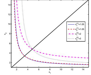
**Fig. 3:** Graphical investigation of convergence of the best response algorithm in the interference limited regime
