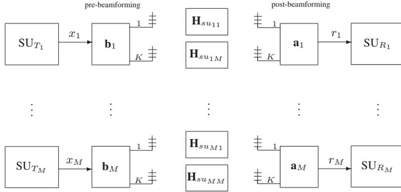
Fig. 1. Multiple transmit and receive secondary users system structure.
