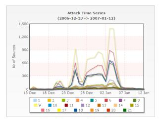
**Figure 4.** The patterns of an extracted clique of attack time series targeting Windows ports and ICMP (I, I-445T, I-445T-139T). Note the almost perfect synchronization of the attacks on 5 different sensors located in 4 different IP subnets.
