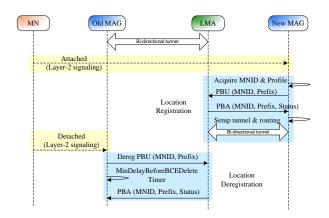
Figure 2. PMIPv6 Sequence Diagram
