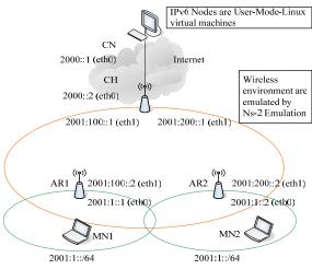
Figure11. Virtual Wireless Mesh Testbed
