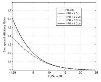
**Figure 6** Sum spectral efficiency gains of the system with one primary user and four CUs
