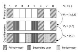
**Figure 2** One primary user and two cognitive users in a spectrum-pooling system with eight sub-bands
