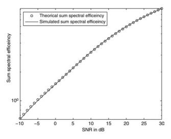
**Figure 4** Comparison between theoretical expression of the sum spectral efficiency in (31) and simulated one in (17) for L = 5 and N = 16
