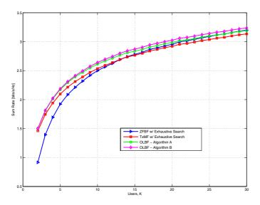
Fig. 2. Sum rate as a function of the number of users for M = 2 transmit antennas, and average SNR = 0 dB.
