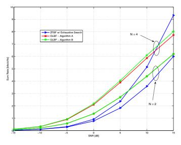
Fig. 1. Sum rate as a function of the SNR for M = 2,4 transmit antennas and K = M users.
