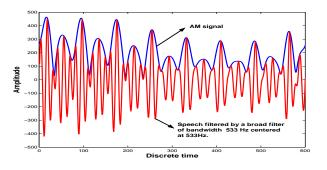
Fig. 3. The AM signal derived using broad-band filters
