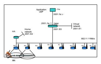
Figure 7: Simulation network topology.
