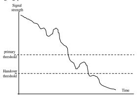
Figure 4: primary and handoff thresholds.
