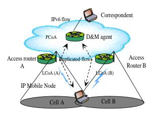
Figure1: IPv6 flow duplication and merging
