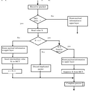
Figure 3: IPv6 flow merging algorithm
